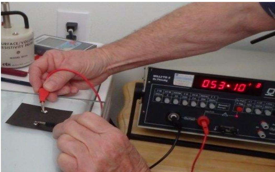
Mercury reading = 5.3E3 Ohms
